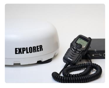
The look and feel is exactly like a legacy LMR system utilizing a simple Push-To-Talk speaker microphone handset. Vehicle installation includes a BGAN on-the-move terminal and an EXPLORER Push-To-Talk (PTT) terminal with a Control Speaker Microphone. Up to two USB modems (optional) can be connected to the PTT base station allowing for two independent cellular network connections. The all important least cost routing functionality enables automatic switching between the available networks:
